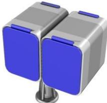
A bifronte outlet tower with four ports, two on each side, mounted on a silver base.        | <p>TORRETTA BIFRONTA A 4 VIE Art.lo: TEUNC.4.10.16.220.44<br/>Corpo: nylon ignifugo ed autoestinguento<br/>Attacco: G 3/4"<br/>Prese elettriche Palazzoli Schuko 10/16A 2P+T 250V IP44<br/>Modello universale con terra centrale e laterale</p> |
