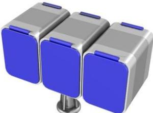
A bifronte outlet tower with six ports, three on each side, mounted on a silver base.       | <p>TORRETTA BIFRONTA A 6 VIE Art.lo: TEUNC.6.10.16.220.44<br/>Corpo: nylon ignifugo ed autoestinguento<br/>Attacco: G 3/4"<br/>Prese elettriche Palazzoli Schuko 10/16A 2P+T 250V IP44<br/>Modello universale con terra centrale e laterale</p> |
